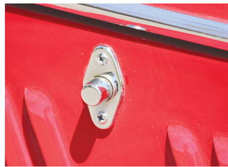
Bonnet release push-button on TF.
