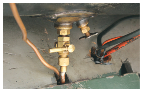
Fuel tap on gravity-fed fuel tank.
