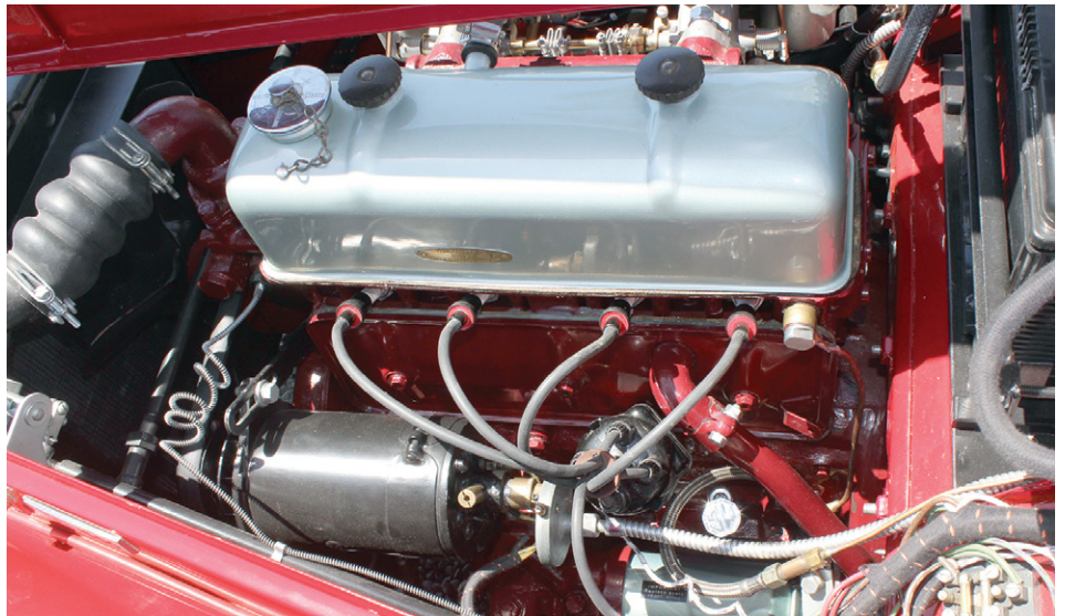
XPEG engine increased the capacity to 1466cc and raised performance around 10%.
