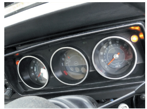
Mini SS dash included extra ignition and oil warning lights.
