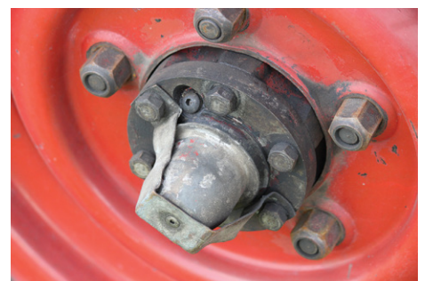
Strap stopped hubcap being knocked off.
