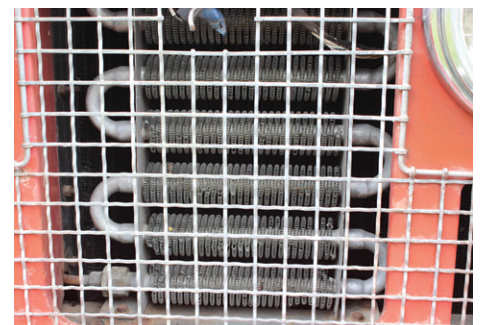
Oil cooler was fitted to fire engines due to the likelihood of static operation.
