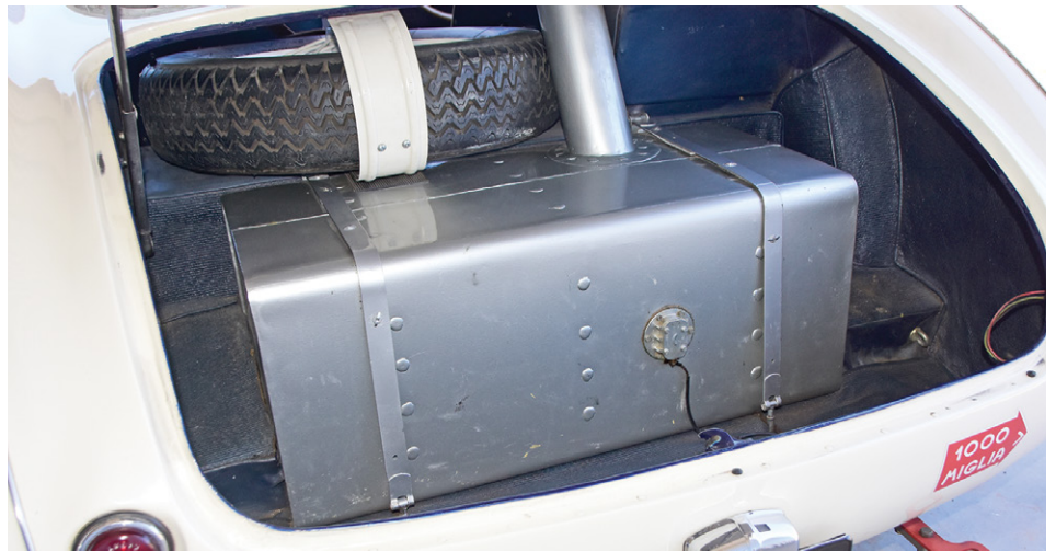
Little room in the boot with 20gal (91lt) fuel tank. Spare wheel moved over to left.
