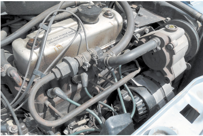
Mini LS engine showing the air pump and plumbing.
