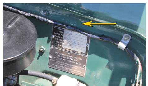
Correct position for Australian ID plates and car number (arrowed) on LH firewall.
