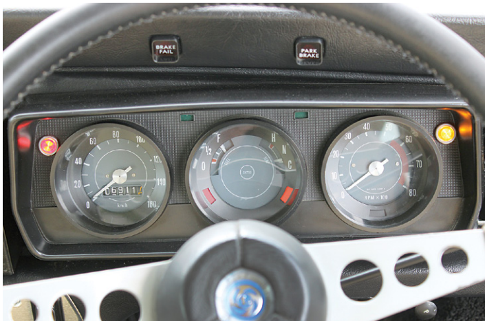
LS dash includes Brake Fail and Park Brake warning lights.
