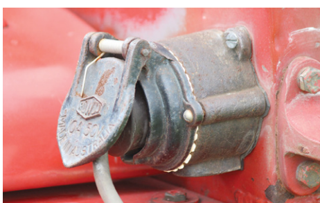
Plug for handheld spotlight fitted in Oz.
