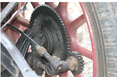
Speedo drive on front-left wheel.
