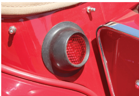
Reflector one of two TF1500 identifiers.
