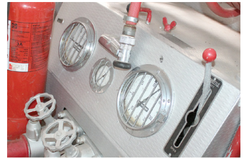
Later units had protective bars over gauges.
