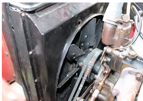
Radiator with wide fan and second fanbelt to avoid cooling system failure.
