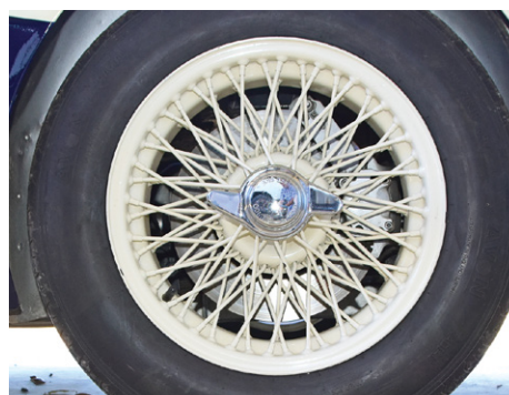
100S had disc brakes on all four wheels.
