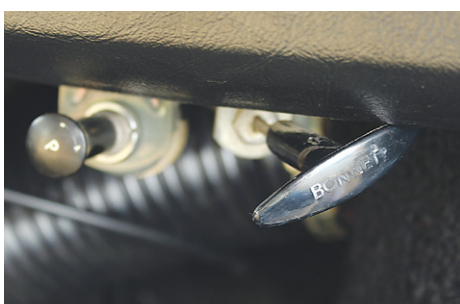
SS and LS have internal bonnet release.
