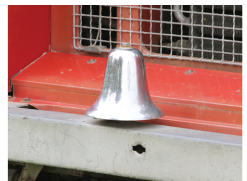
Sirens don't appear to have been on the later SMA units, but electric bells were.
